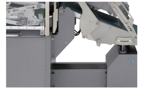
Sloping design prevents dust build up.
